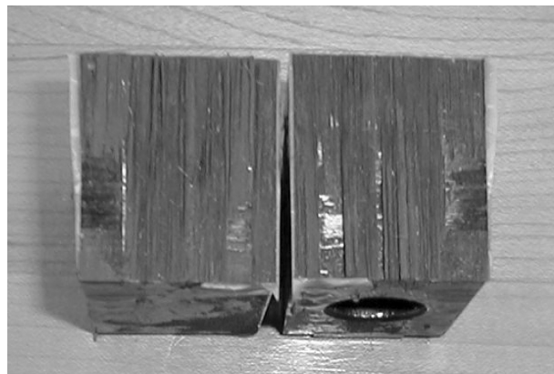
Fig. 4 Transverse tensile test specimen after failure. The failure in this (0,90,0) s specimen is intralaminar.
