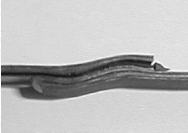
Fig. 1 Side view of wavy joint specimen after failure. The failure is within one of the composite adherends.
