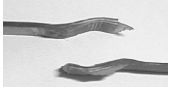
Fig. 3 Side view of tested specimen whose adhesive had not been postcured. No specimens with postcured adhesives failed in the adhesive.
